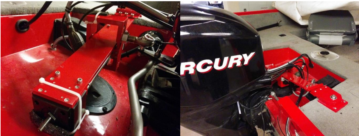
Figure 0-4 Actuator that enables electronic control over the steering
