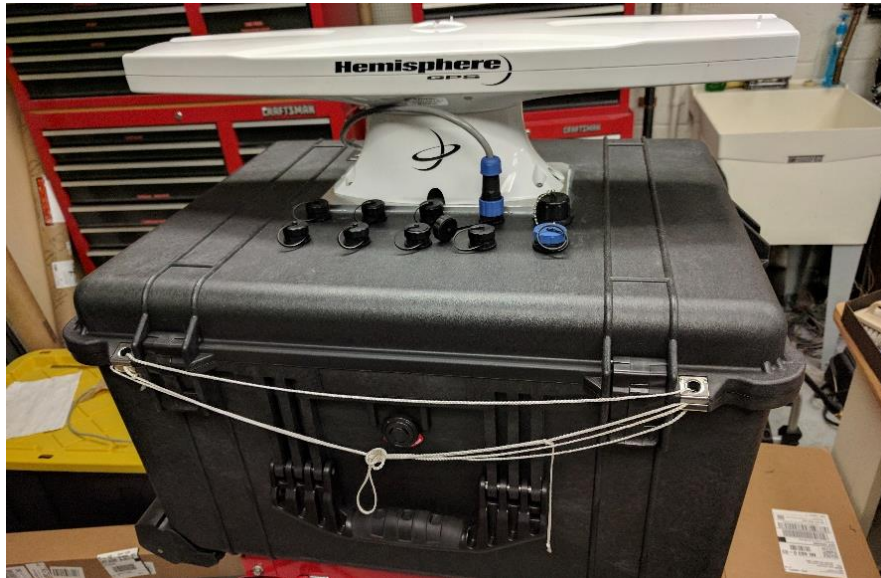
Figure 0-7 Pelican Case with mounted GPS creating a complete autonomy kit
